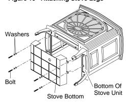
Figure 11 - Attaching Stove Bottom
